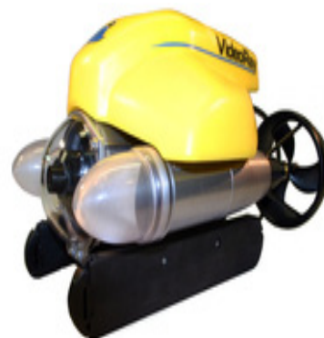
VideoRay ROV (remotely operated vehicle)
